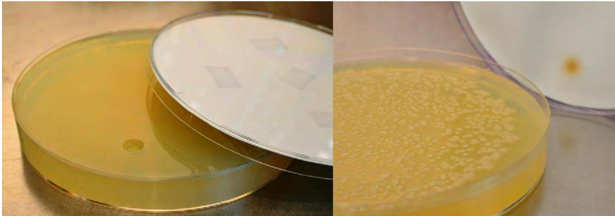
Figure 3: **High-throughput functional screening method for a metagenomic library. Test set-up with positive control in small pit (left picture). Approximately 1.000 clones were tested per 145 mm Petri dish. Detection of an unknown volatile substance causing a brown instead of a blue color change on the filter paper (right picture).**
